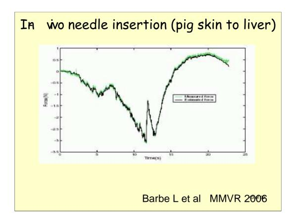
Inserting biopsy needles through skin into liver also takes measureable force, which varies according to the layer being traversed.
