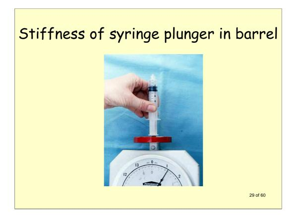
It was very easy to measure how much force it took to push a plunger into a syringe, typically 5 N for a 10 ml syringe and proportionately less for those of smaller size and diameter.
