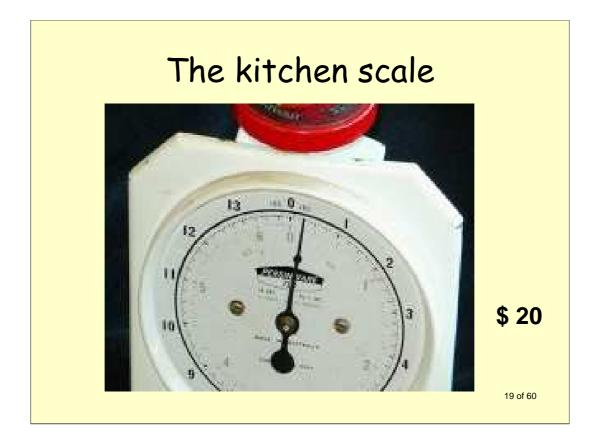
This simple device, a kitchen scale costing a few dollars. Here a tin lid has been screwed in place where the pan usually rests, provides a tool for measuring forces exerted by the hand.
