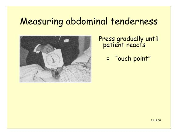
I replaced the pan with a long screw and a cotton reel over which I put a rubber crutch tip. I inverted the scale and reset the reading to zero, because it had changed slightly with the weight of the mechanism pushing the other way.
